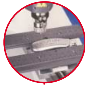
Self-centering vise for easy clamping of objects
